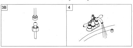
(A) Stainless Steel Braided Faucet Supply . Tubes: This is the simplest of all installations. If you are using stainless steel braided faucet supply tubes, this faucet requires one end of the supply tube to have a 1/2" female IPS connection. The other end of this supply tube must match the thread on the water supply fittings or shut off valve under your sink. Once you have identified the required tube, carefully follow the manufacturer's installations instructions for each tube
