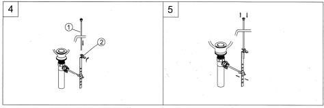
4. Insert lift rod (1) into sink hole, through the linker hole. Tighten the lock nut (2).
