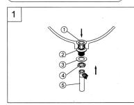
1-1. Remove flange (1) ,rubber washer (2), steel washer (3) and mounting nut (4) from the pop-up
