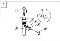
2. Unscrew the nut (4) from the pipe body (6), retain 3. Install the spring clip (1) and linker (2) on the ball the white washer (2), then take off the spring clip (5) from the ball rod (3). Insert the stopper (1), Insert the ball rod into the side hole of drain, slide the nut on and tighten securely.
